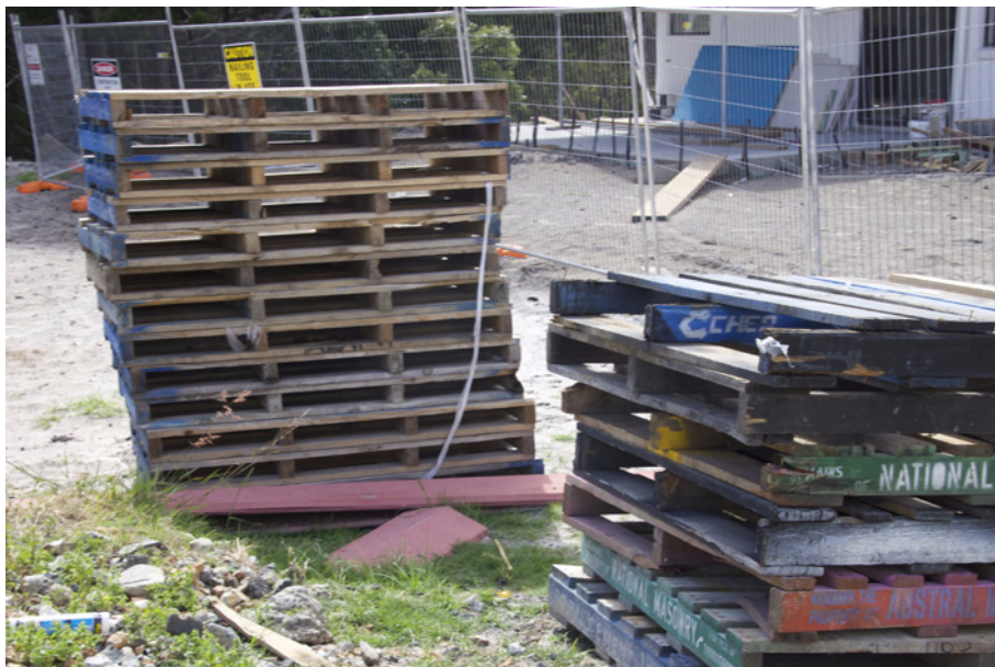
Figure 1-2 Common pallets - the right hand pile is of 1.2 metre square pallets for house bricks. The left pile are pallets for roof tiles. The common industrial pallets are the former. Note the damage and consequent work required to recover even pieces of timber.
